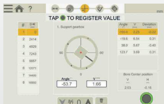
Bore center program, measuring view, first position. Measure 3–50 points at each position (Multipoint). Individual points can be remeasured at any stage.
