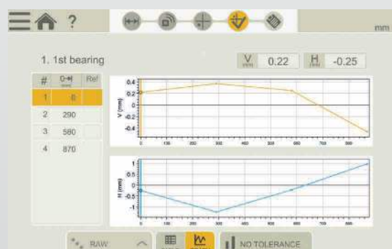
Graph result view. Example with four bores. The result can be displayed as Best-fit calculated.
