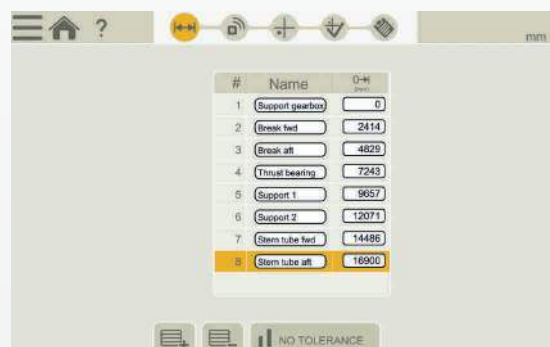
Bore center program, with bores individually named. If required, you can set tolerances.
