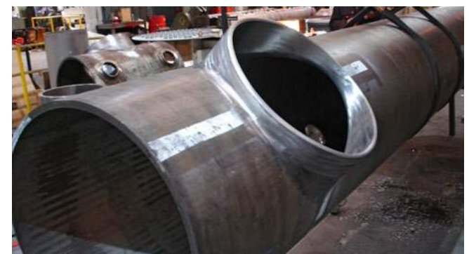
EXTRUDED MANIFOLDS MATERIAL: ALLOY 800HT
