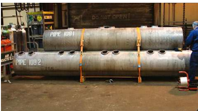
EXTRUDED MANIFOLDS MATERIAL: ALLOY 800HT
